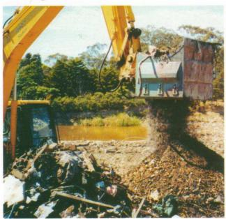
• Designed to suit a range of applications and loader/excavator sizes, the MISU Mobile Integrated Screening Units are available with capacities ranging from 0.3m³ to 3.2m³.
