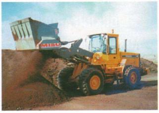
screened using conventional methods. The MISU has proven to be extremely useful for tasks such as screening construction waste from topsoil, which not only prevents the removal of valuable clean topsoil from the site, but also results in significant reductions in waste material transport and disposal costs.
